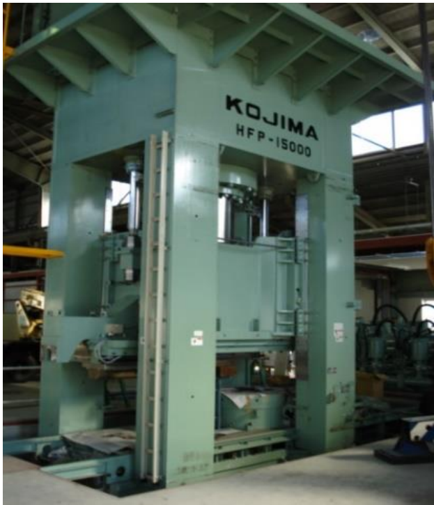
15000kN Hydraulic Forging Press 【Table Size】3,000 × 1,250mm
