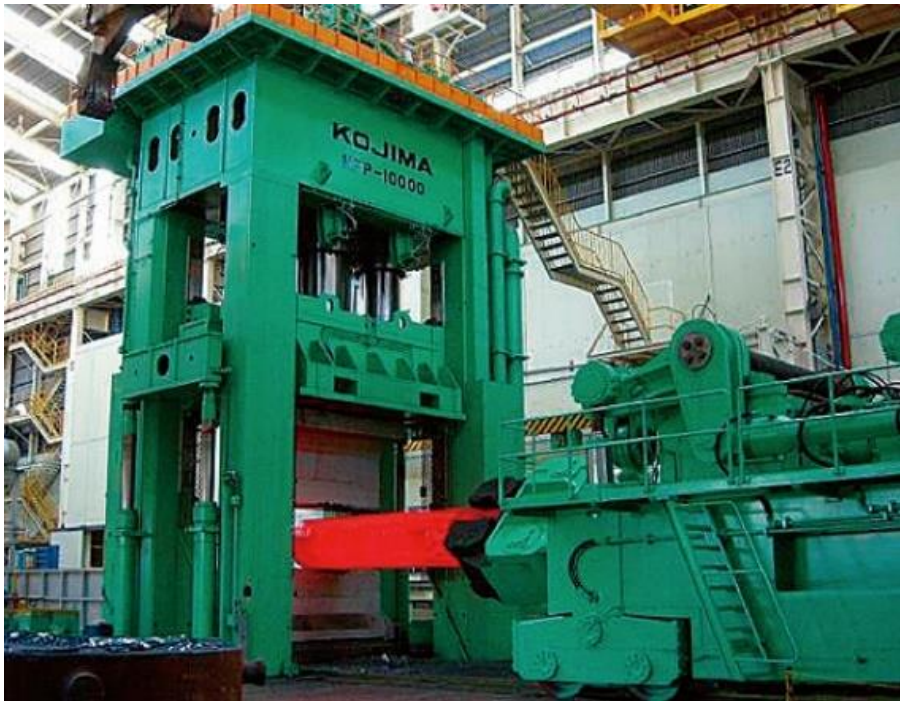
50000kN/100000kN Free/closed Die Hydraulic Forging Press 【Table Size】3,500 × 6,000mm
