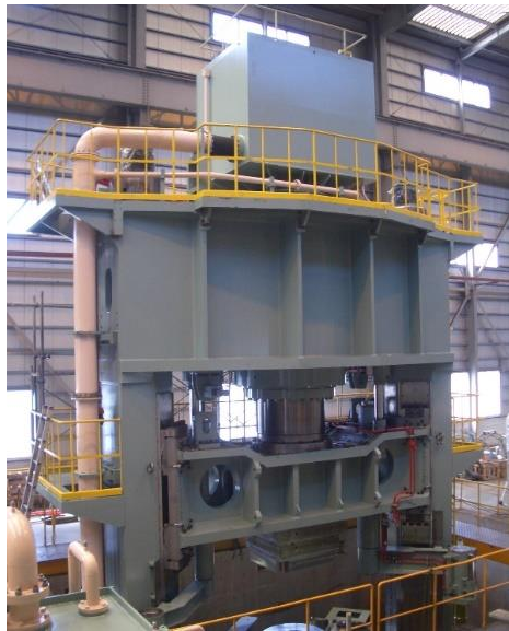
36000kN Two Column Type Hydraulic Forging Press 【Table Size】4,000 × 1,500mm
