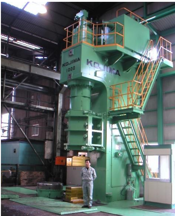
10000kN C-Frame Type Forging Press 【Table Size】4,300 × 1,150mm
