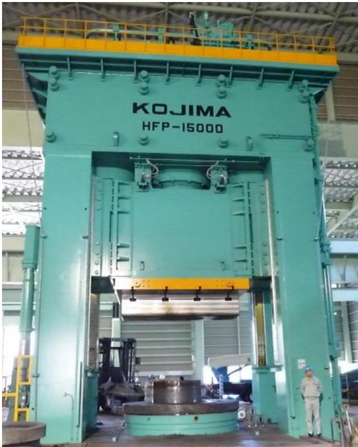
150000kN Free Forging Hydraulic Press 【Table Size】4,000 × 3,500mm
