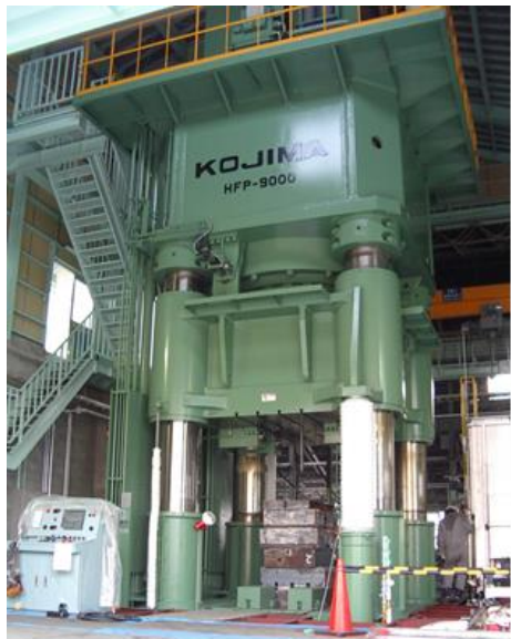
90000kN Closed Die Hydraulic Forging Press 【Table Size】1,800 × 2,500mm
