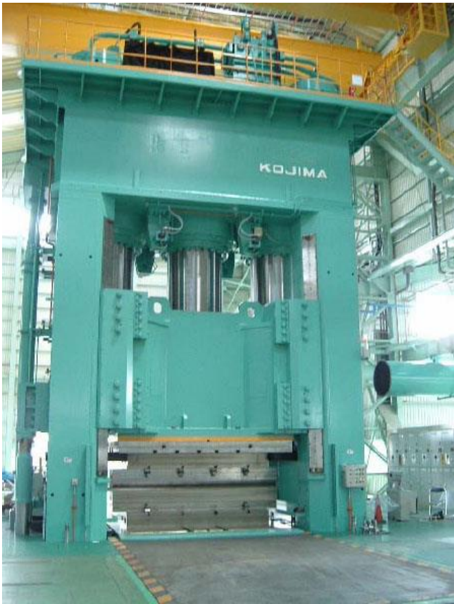
150000kN Free/Closed Die Hydraulic Forging Press 【Table Size】4,000 × 3,000mm
