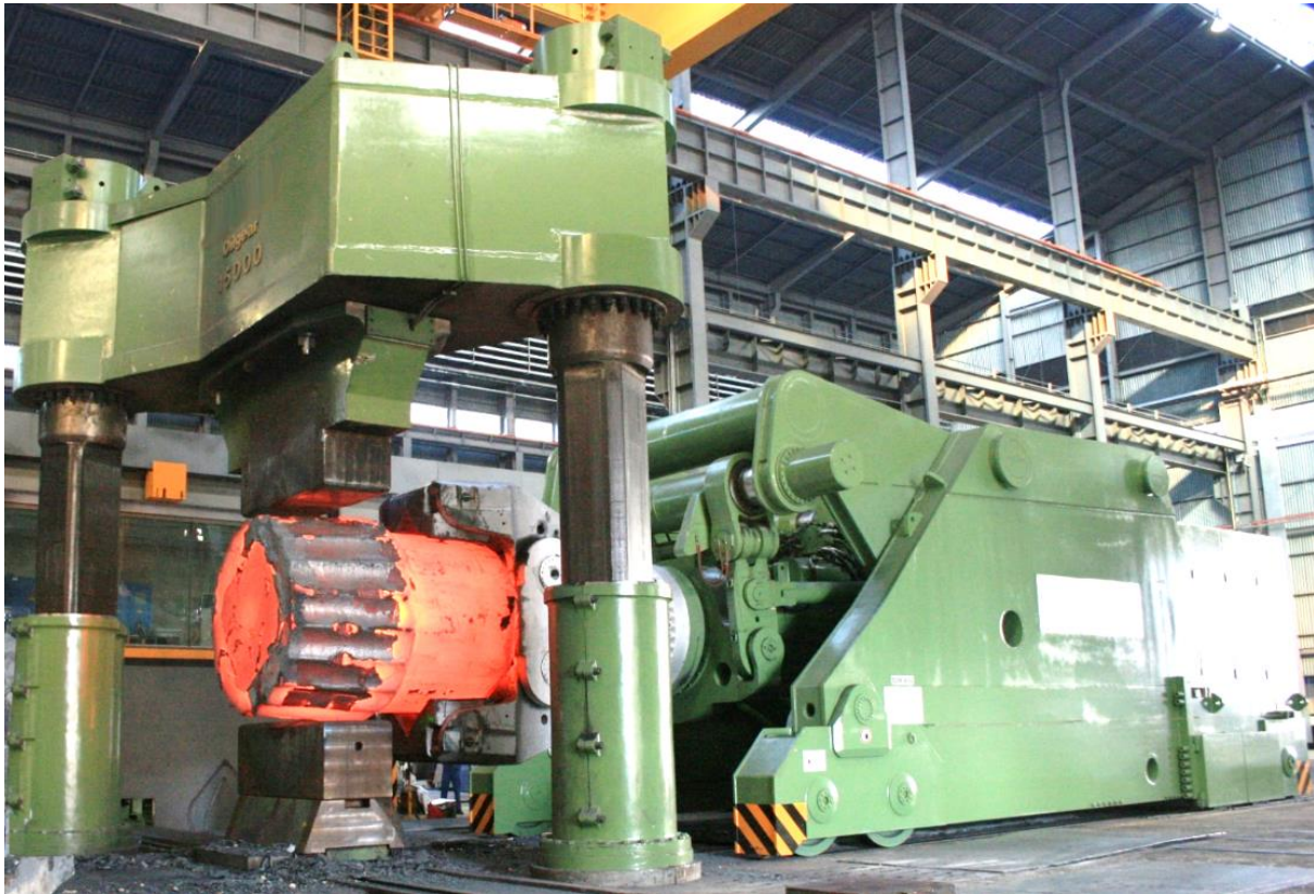
147MN Pull Down Open Die Forging Press 600Bar Hydraulic System 【Stroking Rate】80SPM
