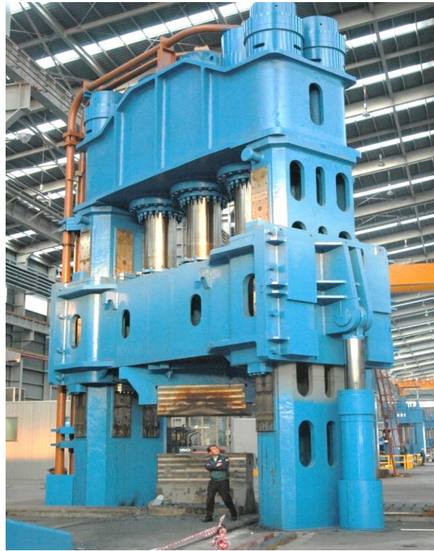
60MN Push Down Open Die Forging Press 350bar Hydraulic system 【Stroke Rate】120SPM 【Positional Accuracy】+/- 1.0mm
