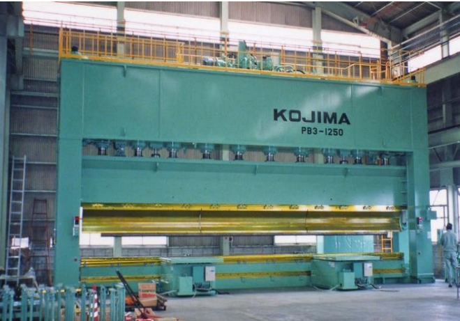
12500kN Long Plate Forming Press with high accuracy Round Columns/Square Columns 【Table Size】11,000 × 520mm
