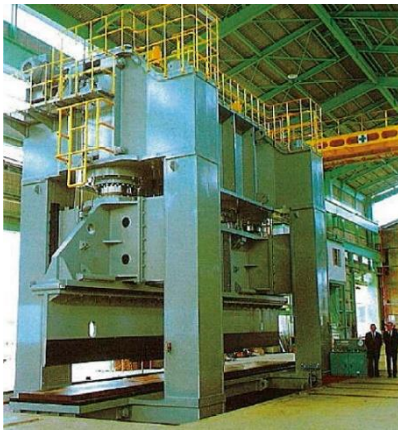
80000kN Long Plate Forming Press Round Columns, Square Columns, Taper Pole 【Table Size】12,200 × 2,000mm
