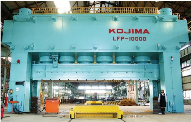
100000kN Hot/Cold Long Plate Forming Press 【Table Size】12,000 × 1,800mm
