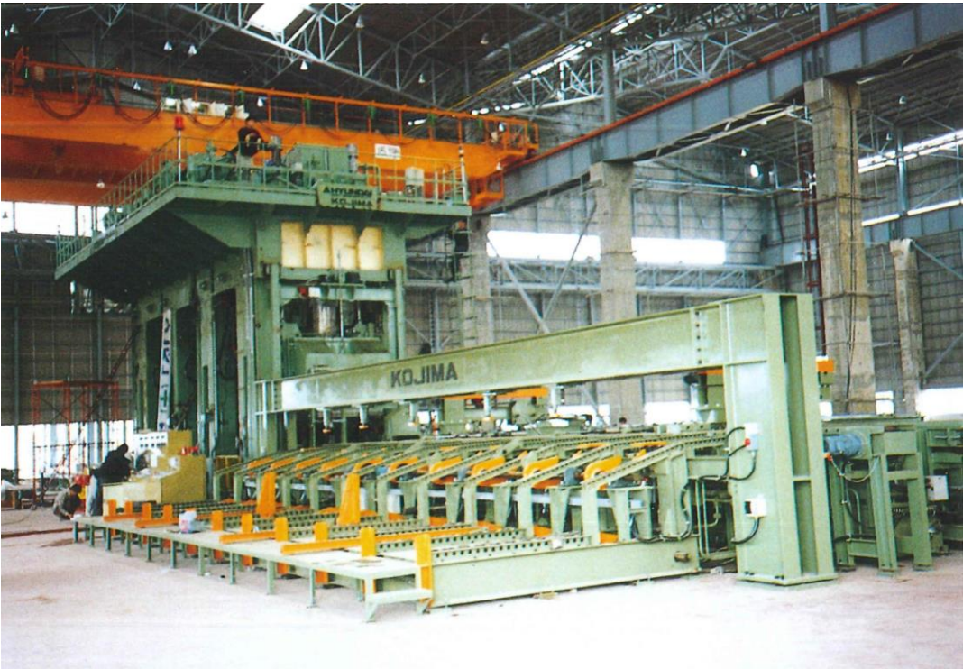
50000kN Chassis Forming Press and Material Handling For Busses and Trucks 【Table Size】 12,000×1,500mm
