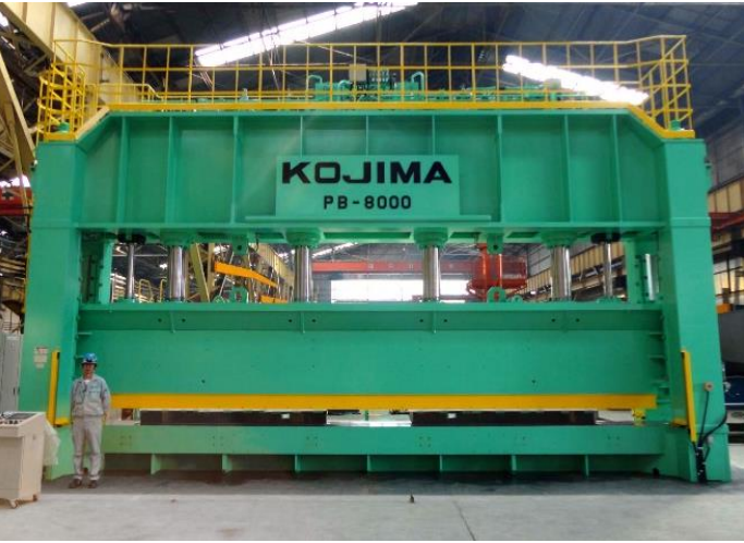
8000kN Long Plate Forming Press 【Table Size】9,200 × 800mm
