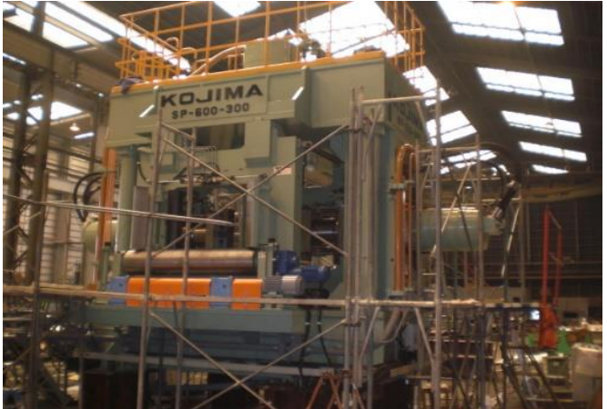
No.5 6000kN X 3000kN Steel Bar Straightening Press (Duplex type)
