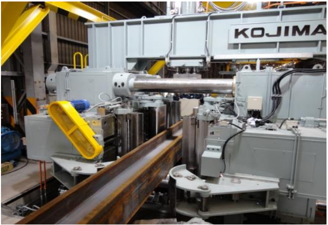
No.4 9000kN Steel Bar Straightening Press 【Main Anvil & Support Anvil distance 】1,450mm
