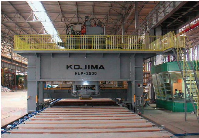
No.2 25000kN Press Leveler with Flatness Gauge 【Table Size】5,200 × 1,000mm
