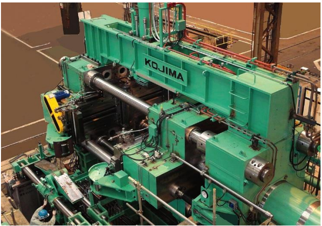
No.3 9000kN Steel Bar Straightening Press 【Main Anvil & Support Anvil distance 】1,450mm
