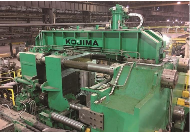
No.5 30000kN Steel Bar Straightening Press 【Main Anvil & Support Anvil distance 】1,500mm
