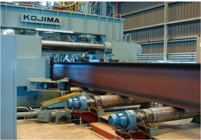
No.2 9000kN Steel Bar Straightening Press 【Main Anvil & Support Anvil distance 】1,450mm
