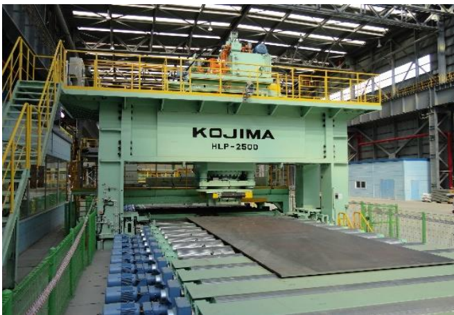
No.4 25000kN Press Leveler with Flatness Gauge 【Table Size】5,200 × 1,300mm
