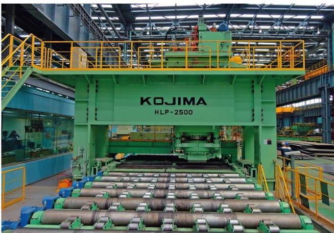
No.3 25000kN Press Leveler with Flatness Gauge 【Table Size】5,200 × 1,300mm
