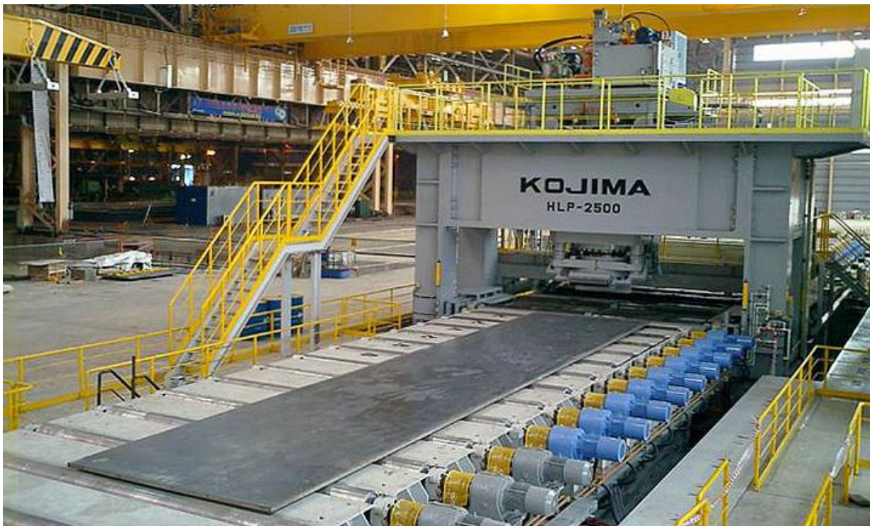
No.1 25000kN Press Leveler with Flatness Gauge 【Table Size】4,500 × 1,300mm
